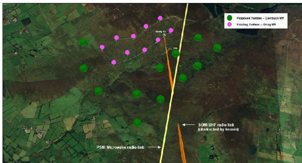
Figure 15. Radio Links crossing through/near proposed wind farm.
